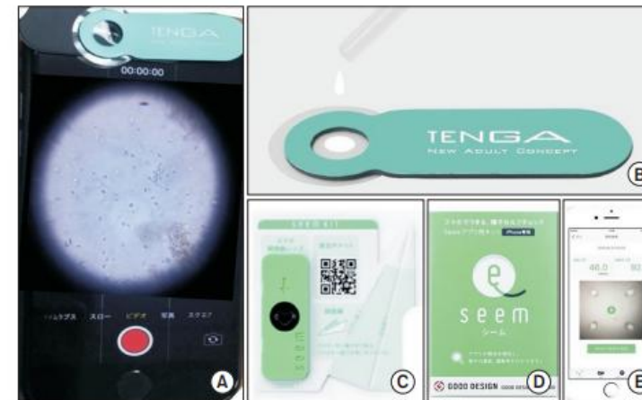
Fig. 4. Men's Loupe (Tenga Health Care) device and smartphone-based SEEM kit. (A) Men's Loupe 0.8 mm diameter ball lens microscope attached to smartphone. (B) Technique for loading semen sample into plastic jacket of ball lens microscope. (C) Magnifying lens semen analysis device with QR code sheet to download the application for operating. (D) Instructions of kit for use. (E) Screenshot of sample test results with concentration and motility.
